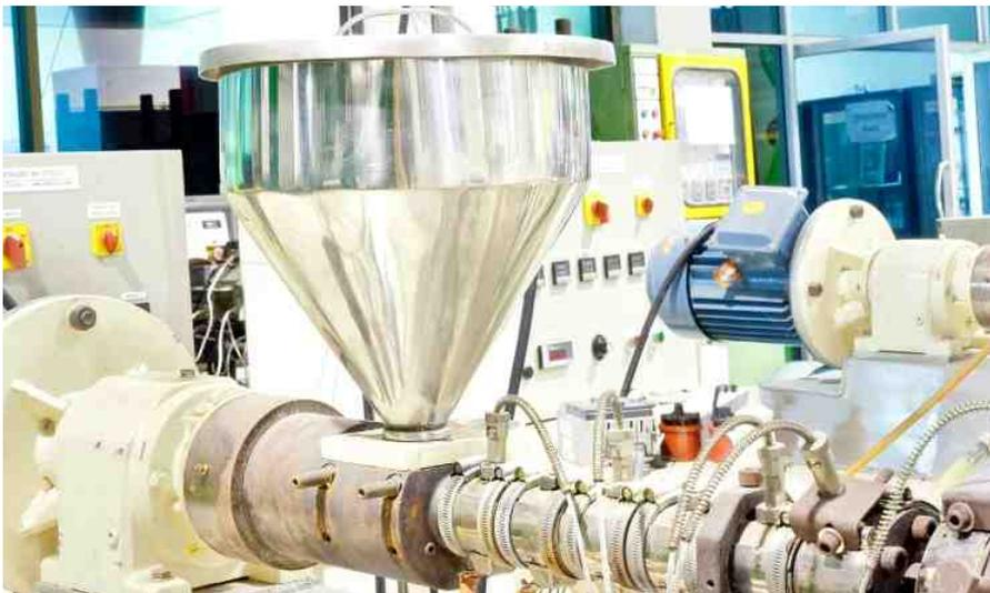
*Excess moisture in plastics decreases product strength and causes a poor surface finish. On the other hand, excessive polymer drying wastes energy and lowers productivity as material delay in the dryer is needlessly prolonged. Dryer dewpoint controls help to achieve good product quality with minimal production costs.*
