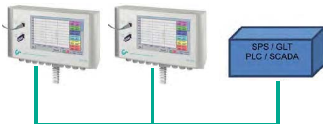
RS 485 network (Modbus RTU) or Ethernet (Modbus/TCP)
