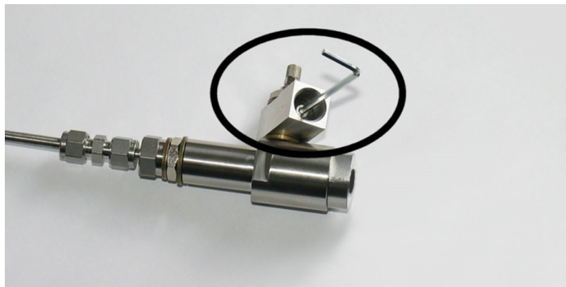
Figure 16 Removing the Leak Screw
