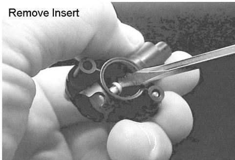
3. As necessary, clean the top of the insert and the inside of the impactor body, to remove accumulated particles.
