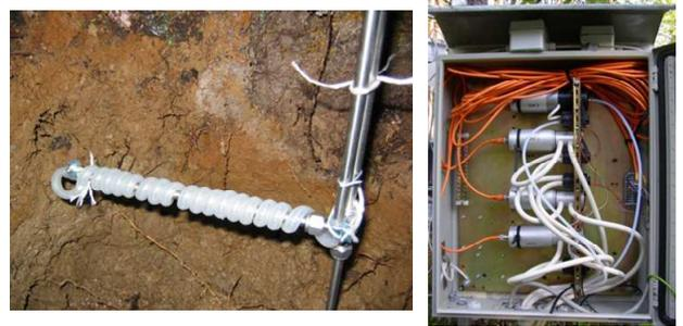
Figure 2. Gas collector installation in the soil (on the left) and the installation box for the GMP343 probes (on the right).
