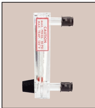
Model MMF mounts easily from front of panel. Drill two 9/32" or 5/16" dia. holes in panel on 2-1/16" centers. Insert mounting connector spuds. From rear, slide on the two spring retainers (furnished) and push on rubber or plastic tubing.
