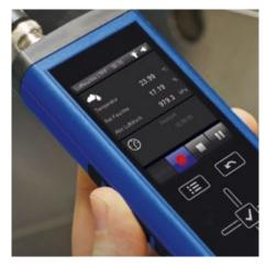
A complete package: the XA1000 is specially engineered for the requirements in the areas of heating/ air conditioning and ventilation to measure temperature, humidity and air flow.
