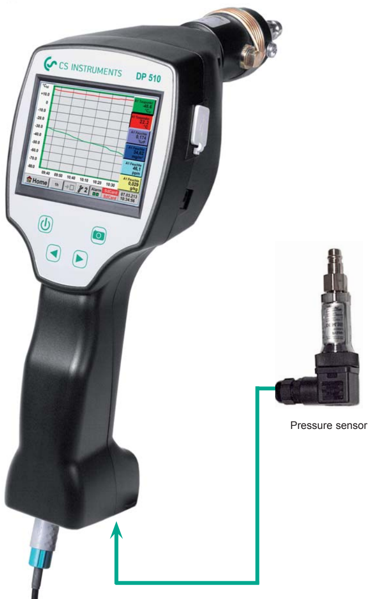
2nd freely assignable sensor input for third-party sensors (only DP 510)
