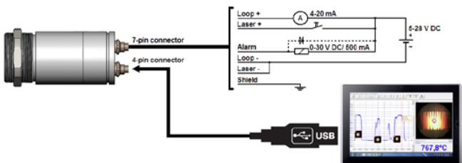
Digital operation mode: process control (Video and temperature) via software
