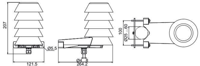
**HMW88/89(D) RH+T and TMW88 T-only transmitters for measurements in wet areas**
