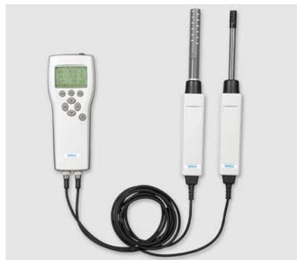
The two ports of MI70 allow measuring CO<sub>2</sub> and RH/T<sub>d</sub> simultaneously
