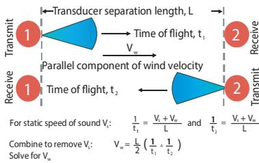
The equilateral triangle configuration of the three transducers provides three possible sets of basis vectors. The combinations yield bi-directional
