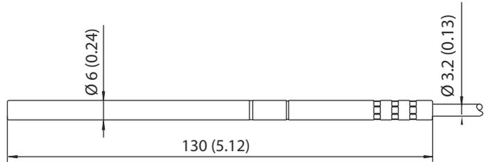
PTU30T for pressure and temperature only measurement
