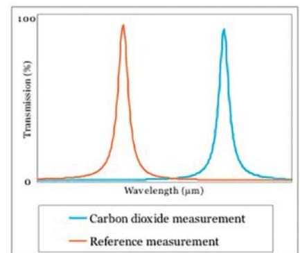
Example of carbon dioxide measurement. Both reference and CO<sub>2</sub> absorption are measured in the same optical path
