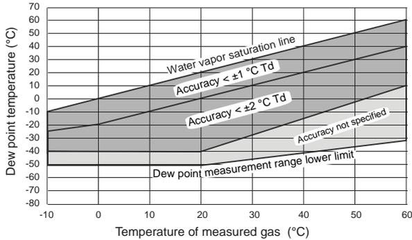
Accuracy (A probe) -40 ... +60 °C  $\pm 2 \text{ }^\circ\text{C}$  ( $\pm 3.6 \text{ }^\circ\text{F}$ ) (see graph)
