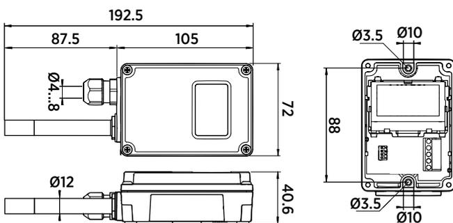
**HMD82/83(D) RH+T and TMD82 T-only transmitters for ducts**
