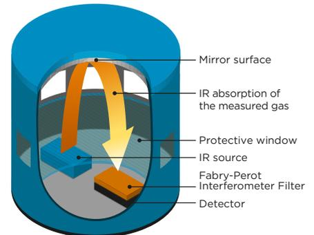
Structure of the CARBOCAP sensor
