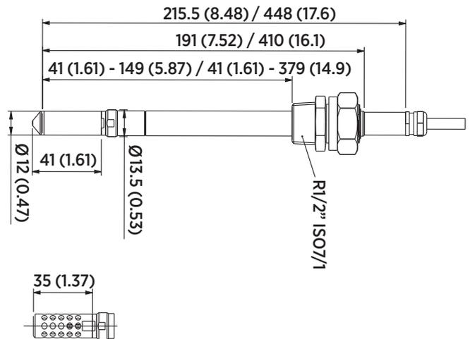
The DMT348 is ideal for installation into pressurized or vacuum processes where the probe needs to be able to be removed while the process is running. The probe depth is adjustable.
