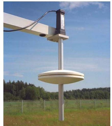
PTB210 paired with SPH10 static pressure head
