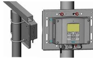
Mounting Rain Shield with Installation Kit
