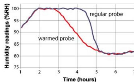
After a period of 100 % relative humidity, the warmed probe measures the true humidity, whereas the non-warmed probe takes time to recover from the condensation.
