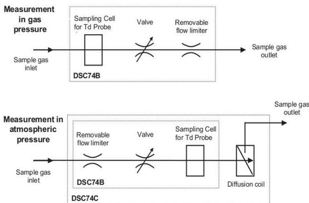
The DSC74B sampling cell enables the measurement of the sampled gas either in gas pressure up to 10 bar or in atmospheric pressure depending on the gas inlet and outlet. DSC74C is like DSC74B but with an additional coil to avoid back diffusion, the effect of surrounding moisture, in dew point measurements in atmospheric pressure.
