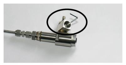
Figure 14 Removing the Leak Screw
