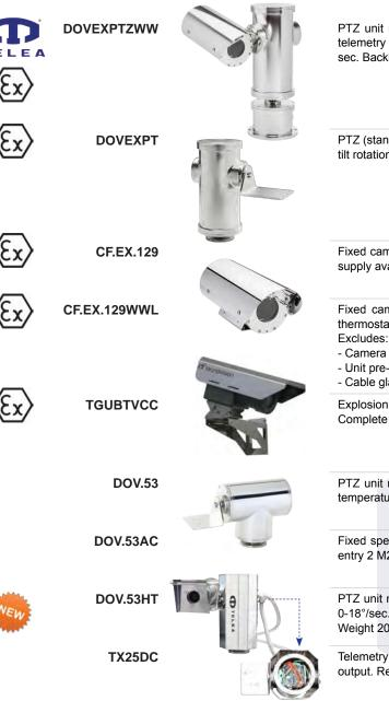
PTZ unit made of AISI316L Stainless steel complete with sunshield, heater and wiper. Protection degree: II2GEx d op pr IIC T6T. Complete with telemetry receiver RS485 Pelco-D protocol. Preset function. Horizontal movement +/-180°, speed 0-18°/sec. Vertical movement +/-90°, speed 0-9.5°/ sec. Backlash <0.1°. Operating temperature: -40°/+55°C. Power supply: 24Vac-95W max. Weight: 25Kg.
