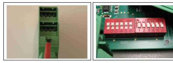
fig. 1: Unscrew housing top
