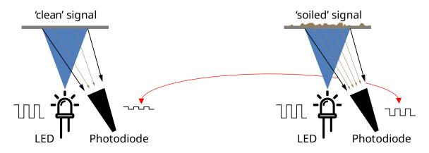
This means that there is a reflected light signal that represents zero transmission loss (0% TL) and there is an uncertainty in determining this value during the factory calibration process.
