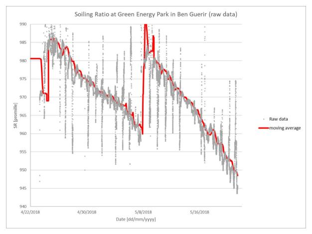
The above sample data shows the data collected in Morocco with daily dew and occasional rain. Still the trendline in soiling build-up is clearly visible.
