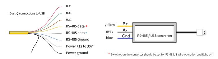
The minimum power supply voltage for the DustIQ instrument is 12 VDC. However, for reliable performance it is advised to **use 24 VDC**, especially when longer cables are used or if DustIQs are daisy-chained.
