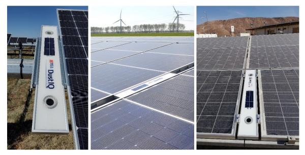
If the DustIQ is installed on a support structure it is advised to use the same end-clamps as you would for 35mm heigh PV modules. The supplied clamps are not meant to be used as an end-clamp.
