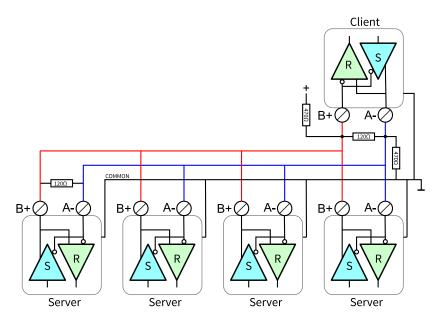
The servers may be a DustIQ, an SMP pyranometer or other 2-wire Modbus RTU device. If this instrument is the last device on the network a line terminator (LT), consisting of a 120  $\Omega$  or 150  $\Omega$  resistor, must be connected between terminals A/A /Data- and B/B /Data+ right at the last device. It is also required to have the pull up and pull down resistors close to or in the client as shown. The value of these resistors must be between 470  $\Omega$  and 850  $\Omega$ .
