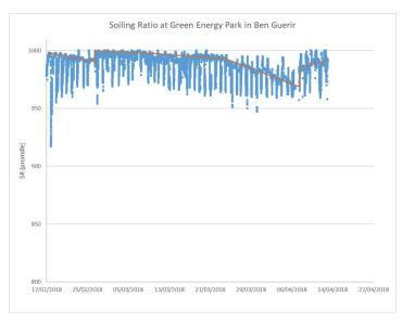
The spikes visible are due to morning and evening dew. The bigger, longer lasting changes are the result of rain cleaning the panel.
