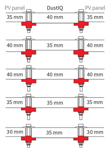
As of serial number 180094 the height of the DustIQ changed from 40mm to a lower 35mm.
