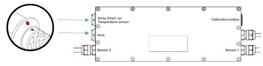
Locate the 8 pin ODU plug correctly in the DustIQ socket, it only fits one way. The red dot on the plug should be opposite of the red dot on the chassis socket. Push it in to secure whilst holding the plug by the end or by the grooved ring.
