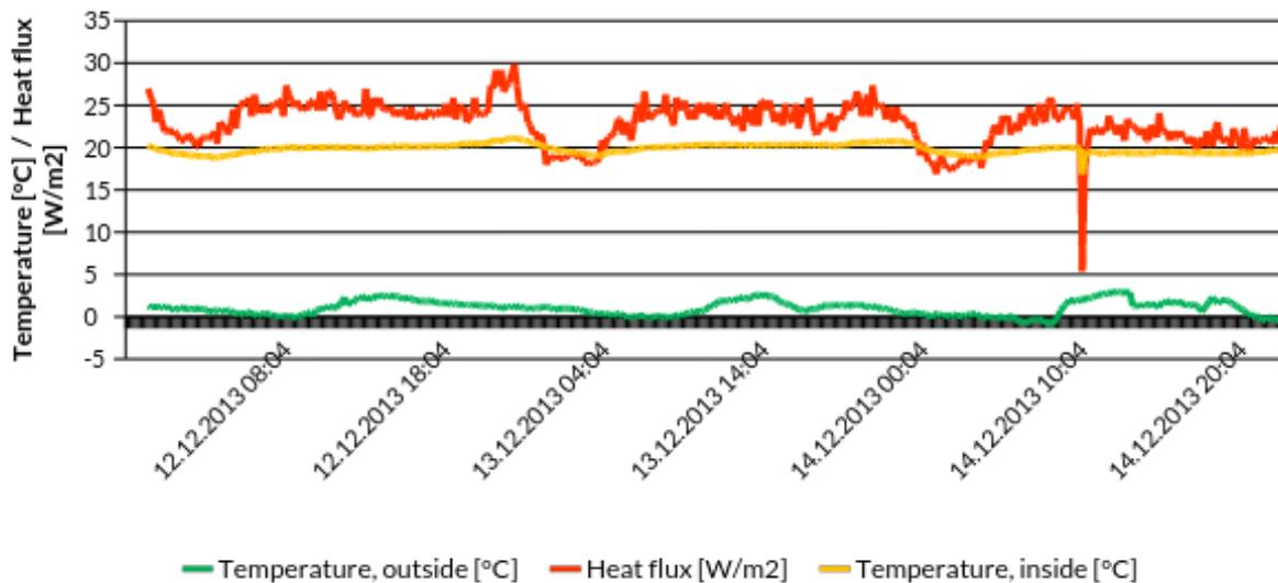
Figure 4. Temperature and heat flux of spot A. This graph was created using the (old) software included in the measurement device (new software version shows directly U-value graph).
