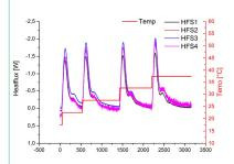
Heat flux response on a series of temperature step. Integration of the peaks yields the energy absorbed by the material.
