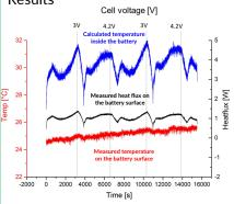
Heat flux (black) and temperature response (red) as measured at battery surface. The temperature inside the battery is
