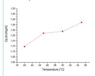
Dividing the determined overall energy by the material mass results in the specific heat capacity
