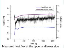
of the battery while applying a temperature difference between top and bottom side. The thermal resistance at steady state condition yielded: 9 W/m/K
