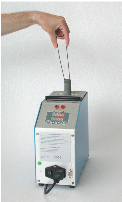
Heating of a probe inserted in a conventional dry-type calibrator.
