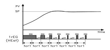
In order to obtain good stability of the temperature, the cycle time "tcr1" has a low value with a very frequent intervention of the control output.
