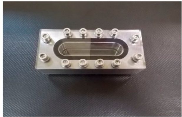
Optical assembly for pressure resistance of 6 Bar. The analysis tank is equipped with Sapphire and Lexan optics.
