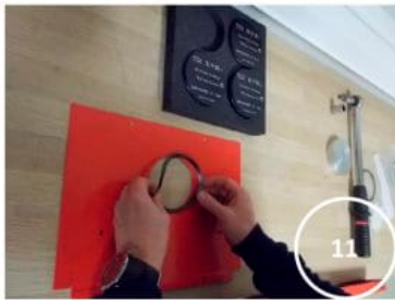
Stick the gasket on the inner side of the cell.
