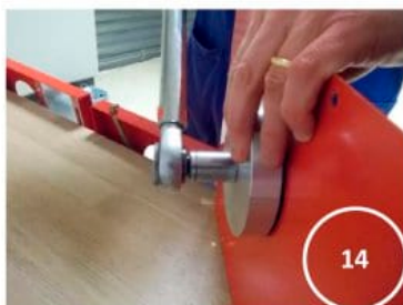
Next, torque with the appropriate key install tool and torque wrench (torque value given on DC).
