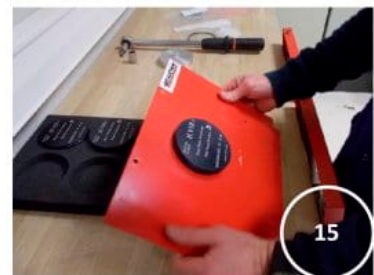
Check the good rotary position, marking must be aligned horizontally
