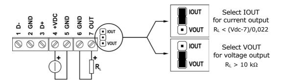
Fig. 3.4: analog output connection
