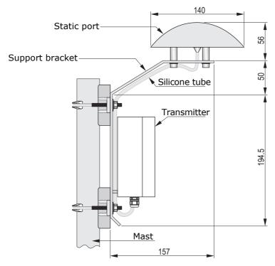
Fig. 3.2: transmitter with static pressure port
