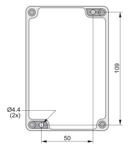
Fig. 3.1: fixing holes
