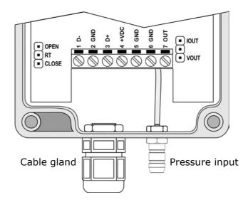
Fig. 3.3: internal terminal header and selection jumpers
