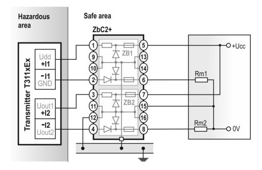
**Warning:** the value of the supply voltage +Ucc must not exceed the value of the maximum allowed working voltage of the Zener barrier (Uwmax = 26 V)
