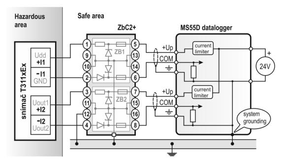
**Warning:** the supply voltage of the datalogger MS55D must not exceed the value of the maximum allowed working voltage of the Zener barrier (Uwmax = 26 V). Use a stabilized 24 Vdc power supply from the recommended accessory (unstabilized ac/dc adapter A1759 is not suitable for power supply).
