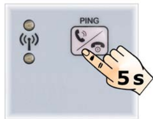
Fig. 3.5: connection button in models in indoor-use housing
