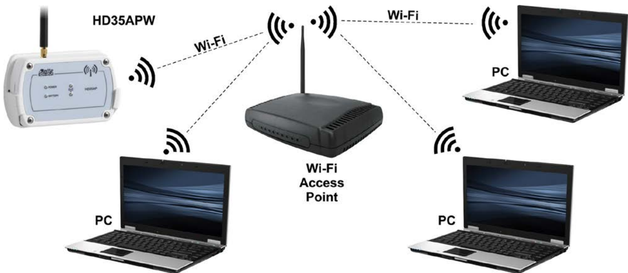
Fig. 6.5.2: base unit in Wi-Fi mode operating as a client
