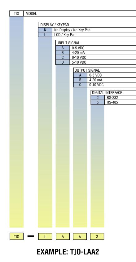
Totalizer I/O Flow Monitor / Controller with LCD Key Pad, 0-5 VDC Input, 0-5 VDC Output and RS-232 Digital Interface.
