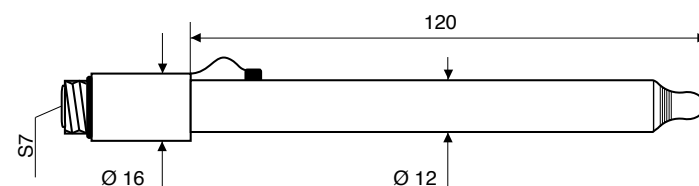
KP90: REDOX PLATINUM electrode, with screw connector S7, reference filling solution KCl 3M, body in glass.
