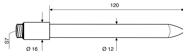
KP 80: Combined pointed pH electrode, gel-filled, with screw connector S7, body in glass.
