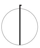
With three sensors in a circular duct, the duct is split into six parts with an angle of  $60^{\circ}$  between.
