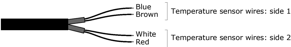
Fig. 6: Connection of probes TP32MTT.03.A and TP32MTT.03.C
