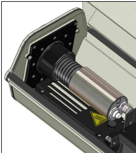
Figure 15: Xi camera mounted in adapter plate
