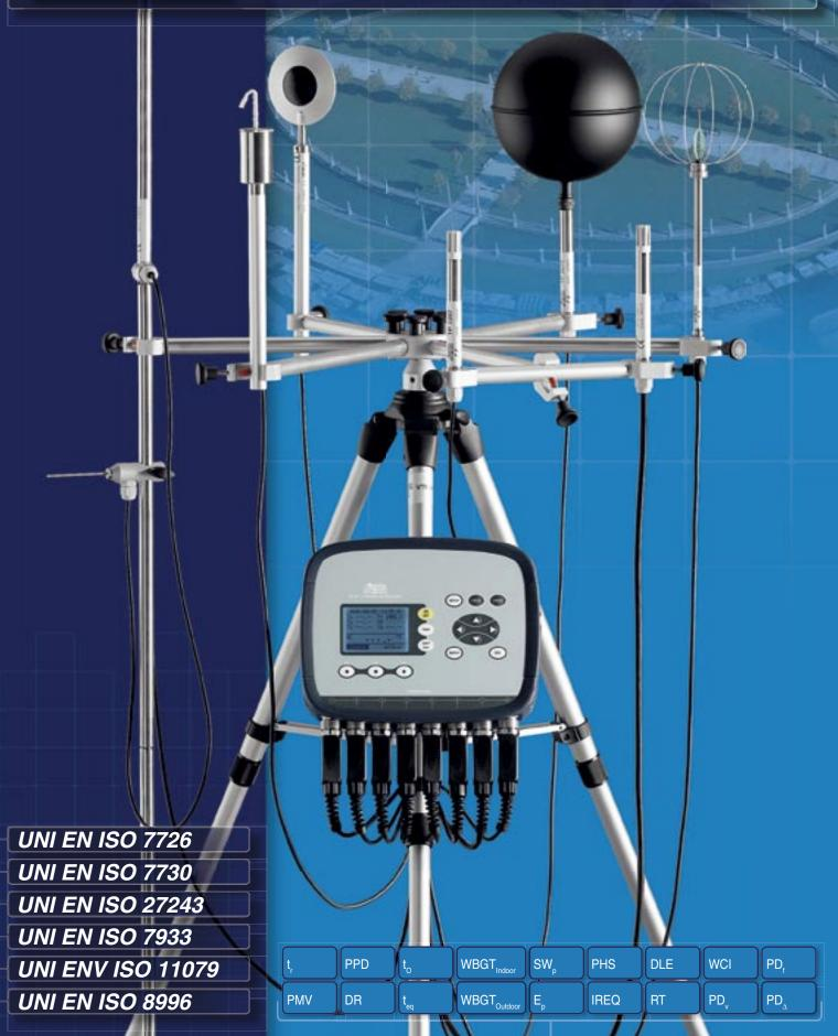
The **Thermal Microclimate HD32.1** instrument is manufactured by **Delta Ohm SrI** and it allows studying, measuring and controlling the Microclimate in the workplace, in compliance with the following standards:
