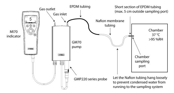
Figure 1 Sampling System with Nafion® Membrane Tube
