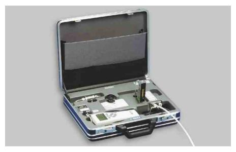
The DSS70A provides a compact solution for field checking dew point where direct measurement is difficult. Typical applications for the sampling system are metal treatment and plastics drying processes.
