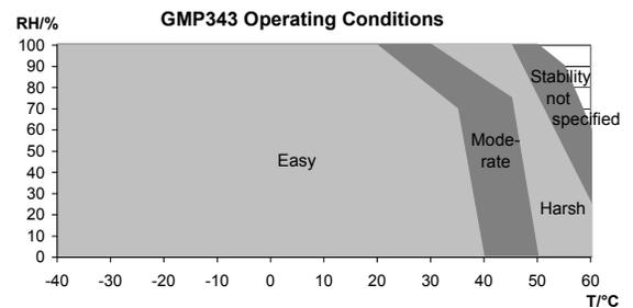
Figure 4. The GMP343 operating conditions.
