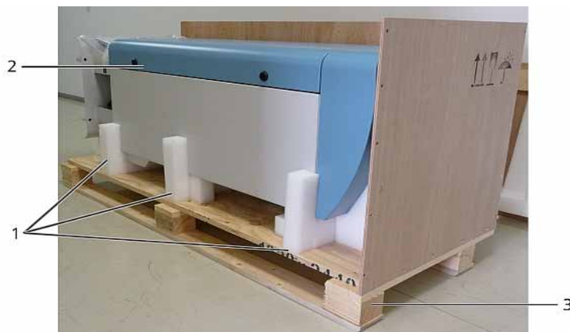
Fig. 6: The CHM 15k with styrofoam packing pads
