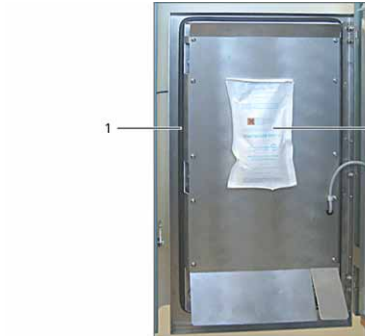
Fig. 28: Air dehumidifier bag (2) and rubber seal (1).
