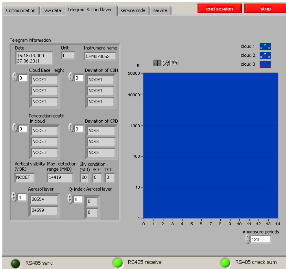
Fig. 32: All types of telegrams contain cloud layer and associated penetration depths; in the advanced and raw data telegrams also the standard deviations of these values and aerosol layers are transmitted. These values are displayed on the left side. The right side shows the course of cloud heights over the last 120 (tbd) telegrams.
