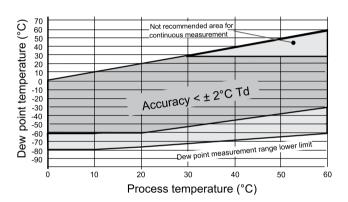
DEW POINT ACCURACY VS. MEASUREMENT CONDITIONS
