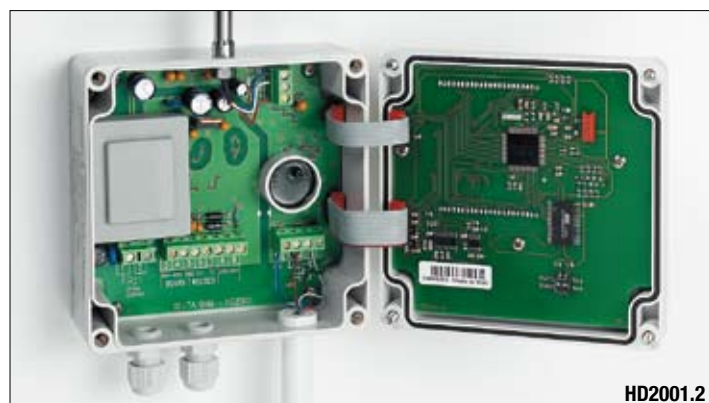
HD2001.2: Temperature, humidity, pressure, air speed, RS232 / RS485 output.
