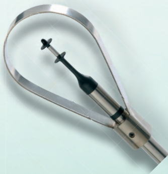
Safety bar Article no. 531 026 To protect the bell head against strong mechanical impacts, it is possible to insert a safety bar made of stainless steel to the sensor tube. This is particularly useful for „clean workbenches“, for example, to avoid unwanted contacts during working. This safety bar excludes any form of aerodynamic impact. Dimensions (W x H x L) : 53 x 11 x 99 mm
