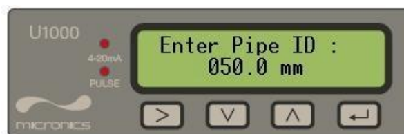
Figure 10 Enter Pipe ID Screen (Metric)
