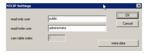
read/write access is only required for synchronizing the clocks, and for transferring camera pictures from a NTCIP station with cameras.
