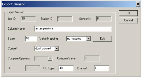
Note for export format "TLS trace file": the sensor values need to be scaled to the appropriate TLS data formats/units (e.g. temperatures in TLS are in 1/10 °C, so they need to be scaled by 10, water film in TLS is in 1/100 mm so they need to be scaled by 0.1 if the "source sensor" is in  $\mu$ m) or converted (e.g. road condition coded in "Lufft def" need to be converted to TLS DE Type 70 coding using an appropriate value mapping).
