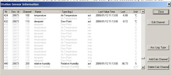
Disabled sensor channels are displayed in gray. For all active sensor channels, the last value time, last value and unit are displayed.
