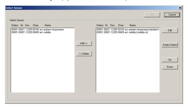
If a station was configured for the export job, only sensors from that station are available on the left side to be selected for the export. A sensor may be selected multiple times. Empty columns can be inserted into the export by clicking "empty column" on the right side.
