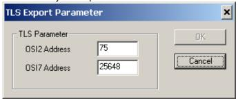
Note: the file that is created by this type of export contains one TLS TC57 (Inselbus) data telegram with "result values" (measure values) for function group (FG) 3 sensors for one timestamp. TLS sensor type and channel assignments are part of the export sensor settings (see below). The values need to be scaled or converted to the appropriate TLS data types or coding as appropriate.
