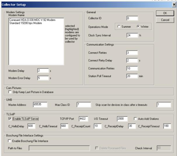
Here you need to select the modem(s) you would like to use with Collector to connect to the stations (if you use dial up connections to your stations). You can assign the modems to different "modem pools".
