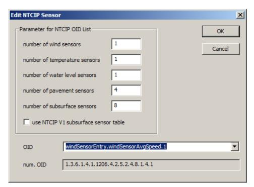
The parameters determine which entries are available in the OID combo box. If the station Meta data has been read from the station, the number of sensor entries for each table is set by the stations actual configuration.
