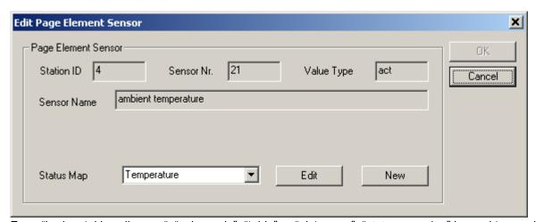
For a "horizontal bar diagram", "color code", "table" or "pictogram", "<u>status mapping</u>" is used to specify which color/text/pictogram is assigned to a specific sensor value.
