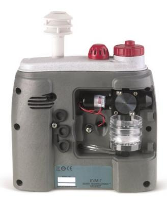
Removal of the back cover allows for convenient access and customization of gravimetric filter cassette for sample collection.
