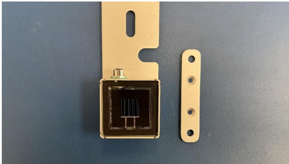
Figure 5-13: Mounting Clean Cell to the dual cell mounting plate
