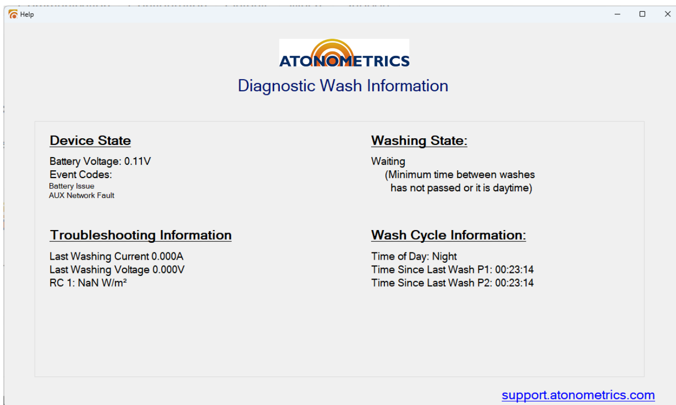
Figure 9-3: Diagnostic Info window showing symptoms of a disconnected battery and disconnected Aux cable
