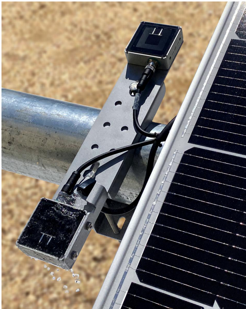
Figure 1-2: A washed and soiled reference cell pair for soiling measurement
