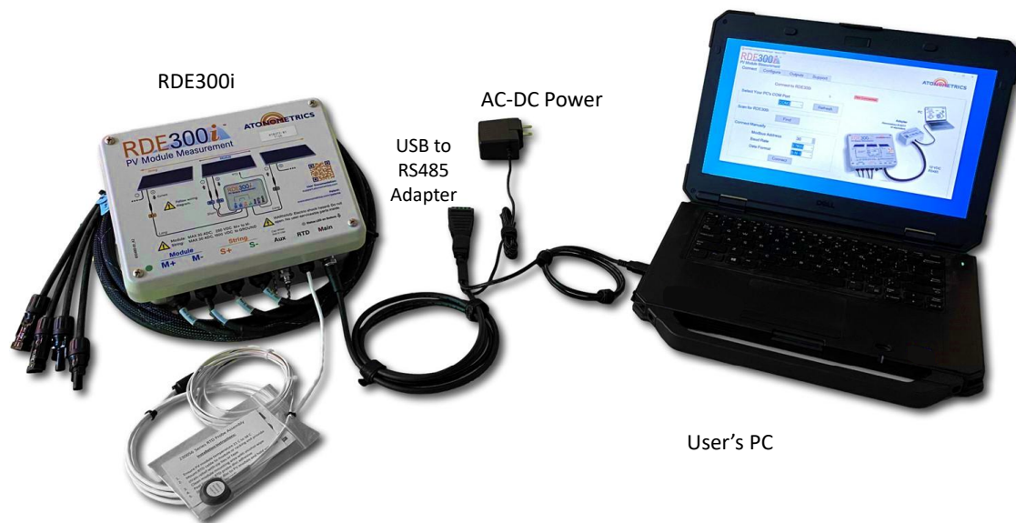
Figure 2-1: Connecting your laptop PC to the RDE300i
