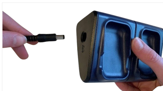
Figure 2-10. Connect PC18 PSU
