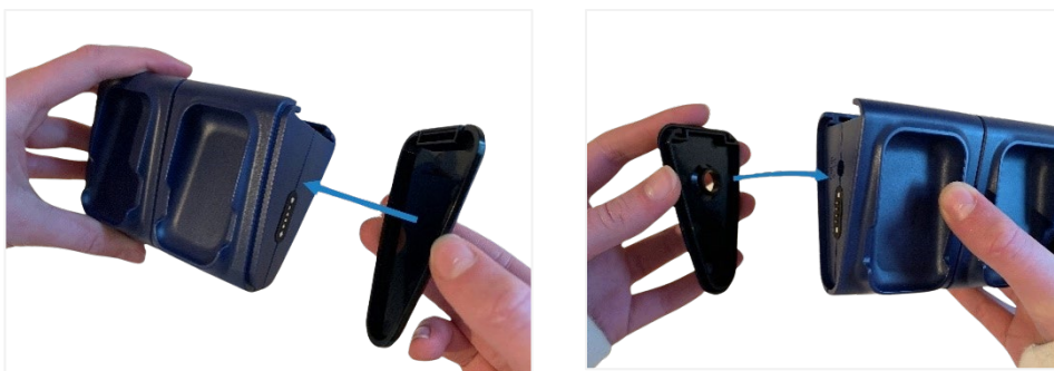
Figure 2-9. Attaching the endplates
