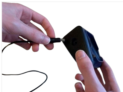
Figure 2-6. Connecting to the charging station
