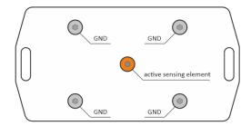
The electrode arrangement ensures reliable detection of water from any direction around the device.
