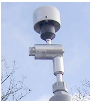
Figure 2-1 Sharp cut cyclone attached to intake
