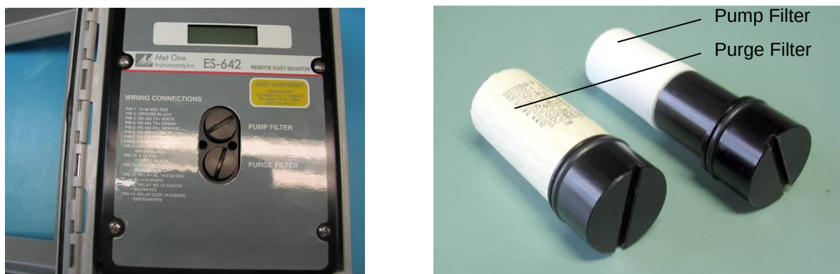
Figure 6-1 Pump Filter and Purge Filter Replacement
