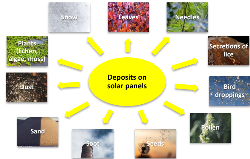
Fig. 5: Types of deposits on solar panels
