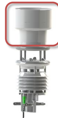
Fig. 10: WS601 with tipping bucket
