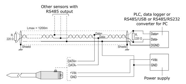
Before connecting the probe to the network, set the address and the communication parameters, if different from the factory preset (see "Setting of RS485 Modbus-RTU parameters" on page 8).
