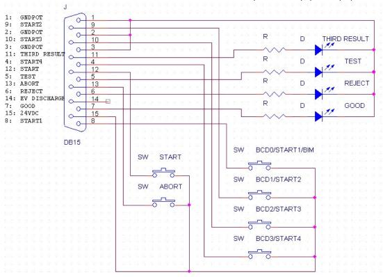
The picture shows a possible complete bench but almost simple, to exploit all the I/O supplied by the connector AUX1 of the equipments M9xxx, M8xxx and M6xxx (in this last case, we remember that pin 4 it is used for the power supply, so the button on the figure doesn't have to mount).
