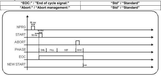
Standard Configuration in case of waste/good with null time:
