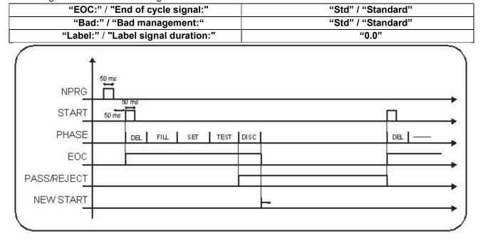
Standard Configuration in case of waste/good with time different from zero:
