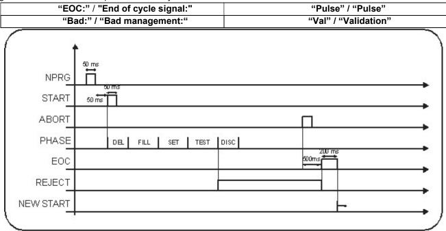
In this case the abort signal serves to validate the test; in fact it decrees the end of the test, the deactivation of waste signal, and the possibility of giving a new start. Since the equipment does not receive the abort signal it remains fixed with waste as result without allowing to make any other tests.
