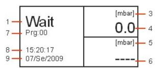
The equipment is waiting when it is not inside a menu, is not under test, does not display a flashing result. There are different possible messages concerning the field 1:
