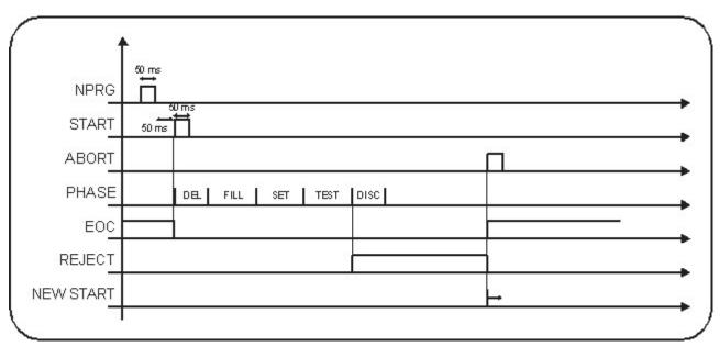
In this case the abort signal serves to validate the test: in fact it decrees the end of the test, the deactivation of waste signal, and the possibility of giving a new start. Since the equipment does not receive the abort signal it remains fixed with waste result without allowing to make new tests.
