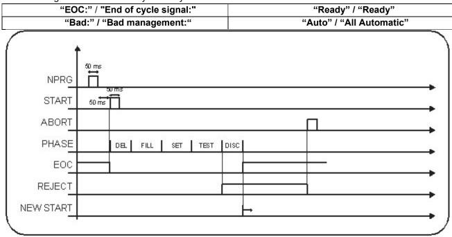
In this case the abort signal serves to disarm waste output, that obviously it would be disarmed also by a new start. In the case "EOC:" / "End of cycle signal:" has the value "Busy" / "Busy" is totally the same, unless that the signal "EOC:" / "End of cycle signal:" has a dual working (i.e. it is low out of the test and high during the test).
