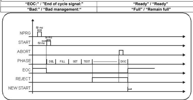
In this case abort signal serves to start the discharge and then to end the test: in fact at the end of the test phase, the discharge does not start in an automatic way leaving under pressure the testing piece (this can be particularly useful in case you want to detect, by soap methods or other ones where is the leak). When the equipment has received the abort signal it starts the discharge phase and the following activations and deactivations of signals.
