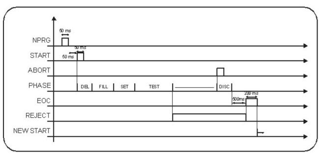
In this case the signal of abort serves to start the discharge and then to end the test phase: in fact at the end of the testing phase the discharge does not start automatically leaving under pressure the testing piece (this can be particularly useful in case you want to detect, by soap methods or other ones where is the leak). When the equipment has received the abort signal it starts the discharge phase and the following activations and deactivations of signals.
