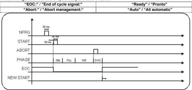
In case "EOC:" / "End of cycle signal:" has a value "Busy" / "Busy" it is totally the same, unless that the signal "EOC:" / "End of cycle signal:" has a dual working (i.e. it is low out of the test and high during the test).
