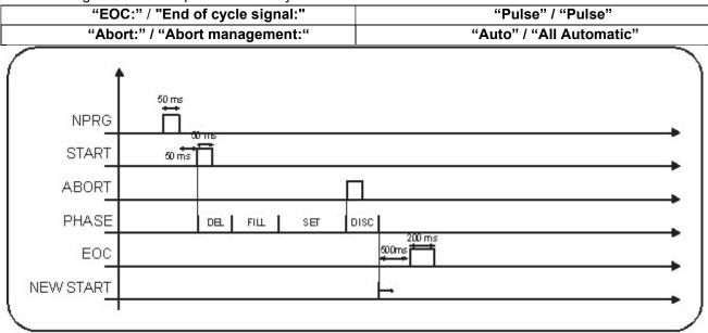
Leak detection configuration with impulsive end of cycle and abort case:
