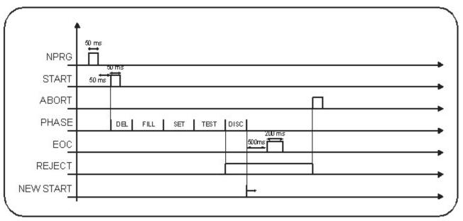
In this case the abort signal serves to disarm the waste output, that obviously it would be disarmed also by a new start.
