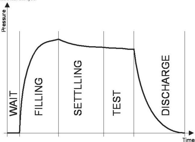
Graphic shows the essential phases of leak test cycle, writing in the graphic the pressure inside the piece. Instead, below you will find the description of all the leak test phases made by the equipment, with the corresponding written message of each phase.
