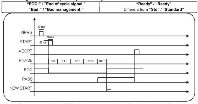
Whatever it is the parameter set "Bad:" / "Bad management:", in case of good as result the behaviour is that one described (it coincides with a waste in case of "Bad:" / "Bad management:" has the value "Auto:" / "All Automatic:"). In the case the "EOC:" / "End of cycle signal:" has the value "Busy" / "Busy" it is totally the same, unless the signal "EOC:" / "End of cycle signal:" has a dual working (i.e. it is low out of the test and high during the test).
