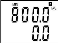
It shows preset value of pressure for voltage output Uout1. Lower LCD line shows voltage value (at V) which is associated to the lowest pressure output (value displayed at upper LCD line). Here 0 V corresponds to 800 hPa.
