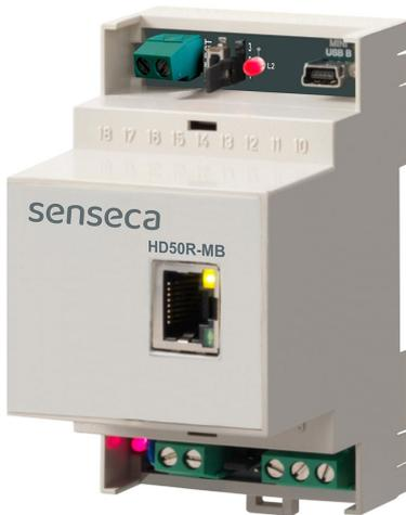
Data logger with **Master** RS485 Modbus-RTU interface for acquiring sensors with RS485 Modbus-RTU output (for example an anemometer of the HD52.3D... series). A voltage-free contact input allows connecting a rain gauge with contact output.
