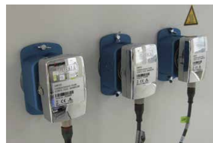
Figure 2. GMP231 probes installed for the heat sterilization test. The PTFE filter covering the sensor head and the silicone installation plug can be seen in the inside view (left). The outside view (right) shows the wall feed-through.
