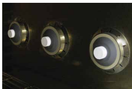
Figure 2. GMP231 probes installed for the heat sterilization test. The PTFE filter covering the sensor head and the silicone installation plug can be seen in the inside view (left). The outside view (right) shows the wall feed-through.
